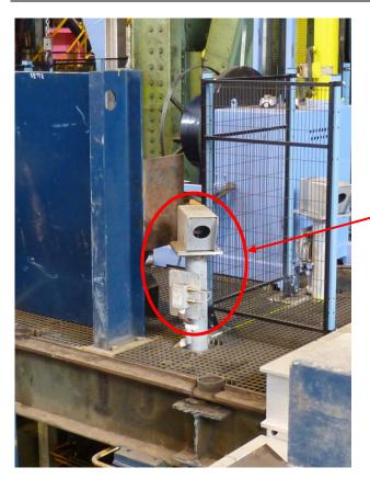
Retro-reflective barrier LRD 600 with optics OADF 104 and fiber glass cable LLK 2
