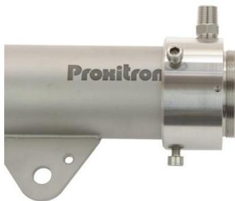
PROXITRON diffuse sensors can be provided with an additional air purge to protect the optics from contamination. The recommended operating pressure is 0.15 bar. This value corresponds to a consumption of 60 liters/min. The maximum operating pressure is around 0.3 bar. The scavenging air must be oil-free, dry and dust-free in order to prevent contamination of the optics. For optimum performance of the air-purge unit to use an additional protective tube OL 37 or OL 38 is recommended.
